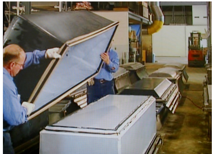
The plastic liner is also coated with resilient adhesive before being joined to the metal
