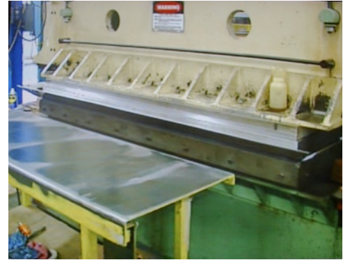
Sheets of 26 gauge stainless steel are inspected, cut and stamped
