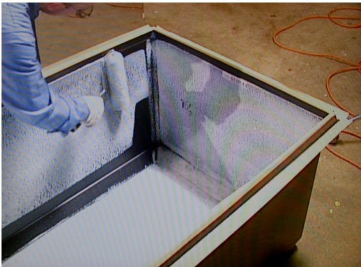
The plastic liner is also coated with resilient adhesive before being joined to the metal
