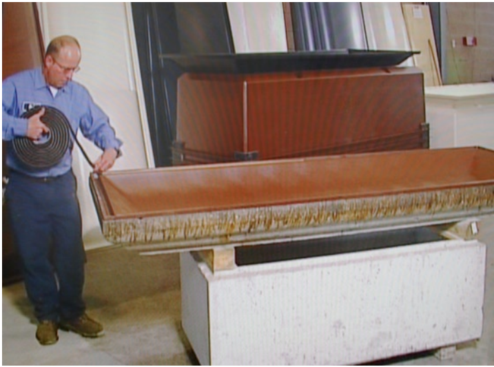
Butyl tape is installed in the cover. This will seal the cover to the base
