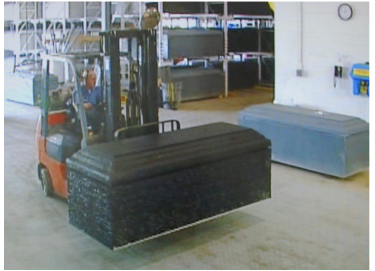
The vault is basecoated and then stored until it's fully cured and ready to use
