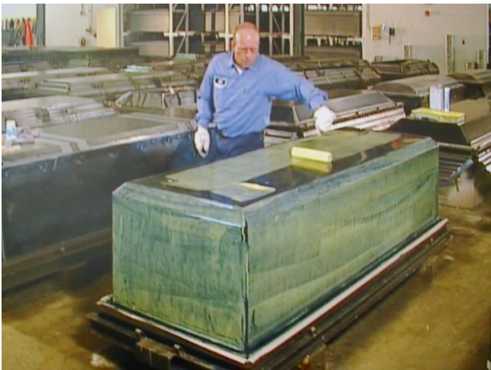
Wilbert's patented Unidex epoxy is applied to the outside of the plastic liner which will bond the liner permanently to the concrete
