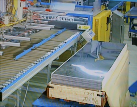
Sheets of 26 gauge stainless steel are inspected, cut and stamped
