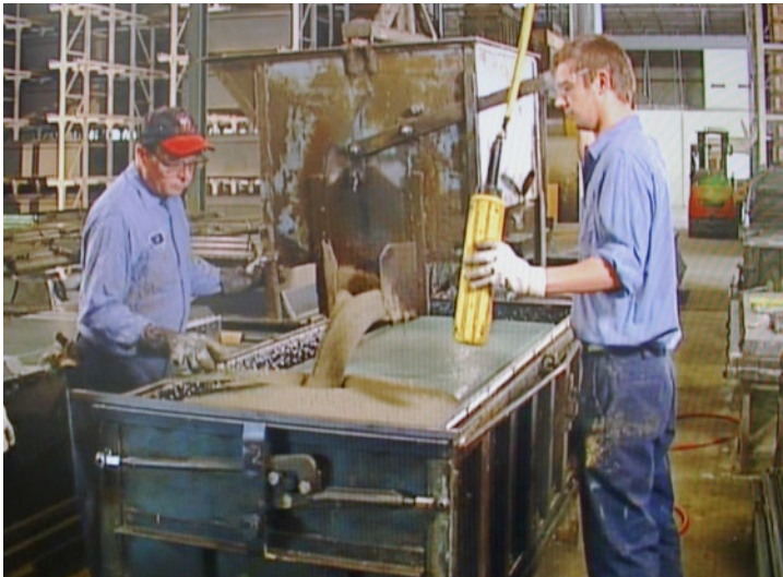
Concrete is poured into the mold
