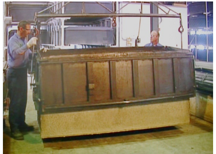
The next day the vault is removed from the mold
