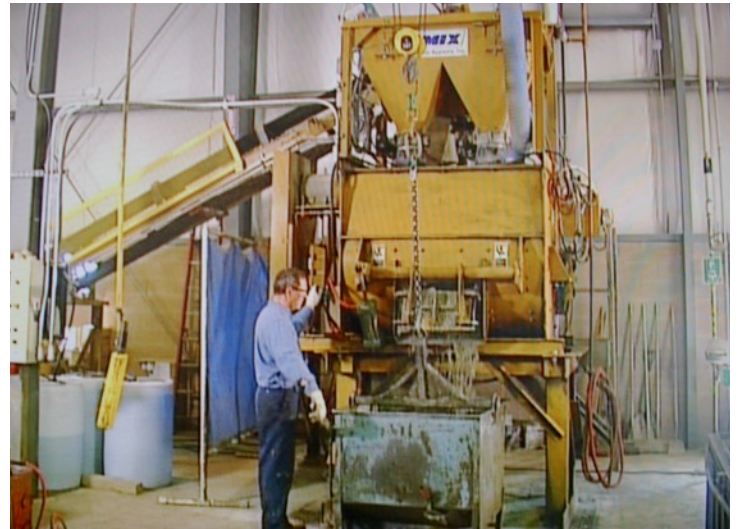
High strength concrete is mixed Note: our concrete surpasses 6,000 psi, the concrete found in sidewalks and roads is typically around 3,500 psi
